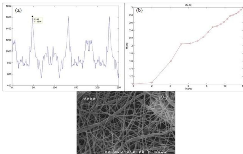
**Figure 2: a) Diagram of Angular Power Spectrum, b) Graph the Movement Curvatures of Nanofibers between Nozzle and Collector and c) SEM Image of PCL Nanofiber in Field Switching 0.2 second**
