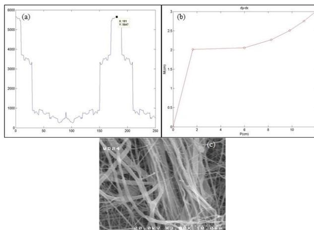
**Figure 4: a) Diagram of Angular Power Spectrum b) Graph the Movement Curvatures of Nanofibers between Nozzle and Collector and c) SEM Image of PCL Nanofiber in Field Switching 0.4 Second**
