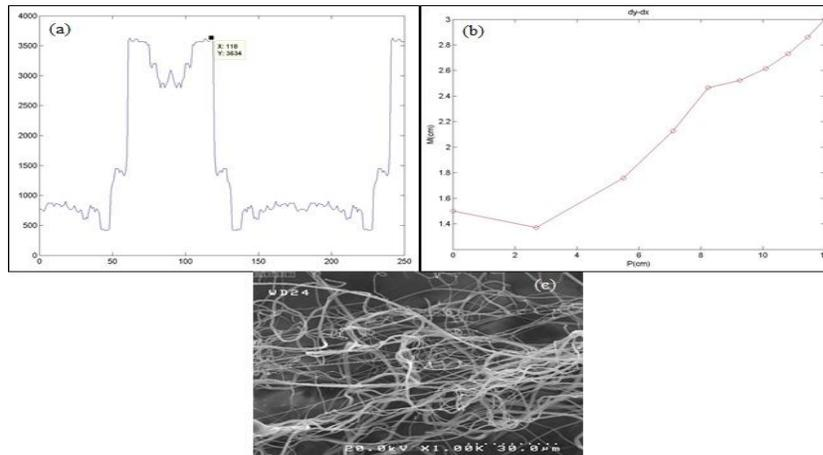
**Figure 3: a) Diagram of angular Power Spectrum, b) Graph the Movement Curvatures of Nanofibers between Nozzle and Collector and c) SEM Image of PCL Nanofiber in Field Switching 0.3 Second**
